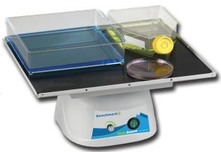
The Orbi-Blotter features a gentle orbital motion with speed control down to as little as 3 rpm, making it the ideal orbital choice for low speed applications, such as blotting, washing, staining/destaining, etc. A large 14x12 in. platform is included along with a non-slip rubber mat for holding trays, dishes, plates, flasks and other flat bottomed vessels. An optional stacking platform is also available for protocols requiring an increased work surface.
