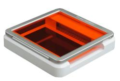
The UltraSlim LED illuminator is designed for viewing stained gels on the laboratory bench, or within gel documentation systems. The dimensions is only  $210(W) \times 210(D) \times 30(H)$ mm. Lighting from the LED source inside the instrument produces blue light with a narrow emission peak centered at approximately 470 nm, which is more effective for the excitation of most nucleic acid and protein stains
