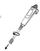
③ Separate the seal gasket and O ring from piston cover.
