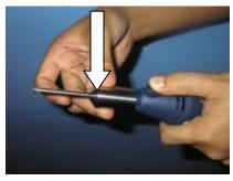
7. Press the black locking button and screw it fully onto the drive!
