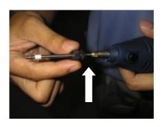
5. Put collette lock head onto the shaft and srew it back to the drive itself! While doing that you must press the black button to lock it.
