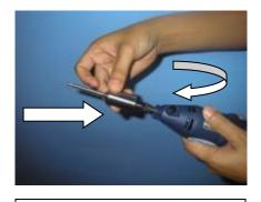
6. Put the shaft tube onto the axle and screw clockwise onto the housing!
