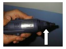
1. Hold H100 drive open the collette and press the black button to lock it and unscrew the collette.
